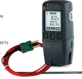
This standalone data logger measures and stores more than 250,000 temperature readings from two K, J or T-type thermocouple probes at a resolution of 0.1°C (0.2°F). It comes supplied with two K-type thermocouples capable of measuring from 0 to 200°C (32 to 392°F).
