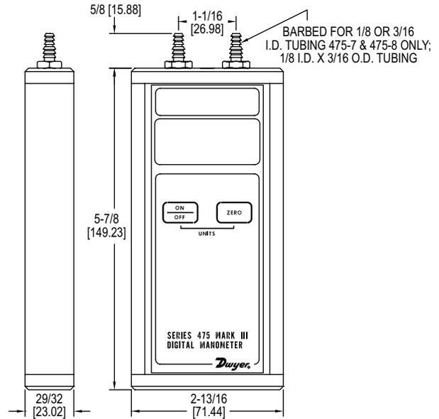
The **Series 475 Intrinsically Safe Handheld Digital Manometer** measures positive, negative, or differential pressures of air and natural gases in ranges from 1 in w.c. (0.249 kPa) to 150 psid (10.34 bar). The dual push pads on the front panel control the on/off, auto zero, and pressure unit selection, allowing for simple operation with no set up needed. When used with a Dwyer® Pitot tube (●), the Series 475 can also be used as an air velocity gage.
