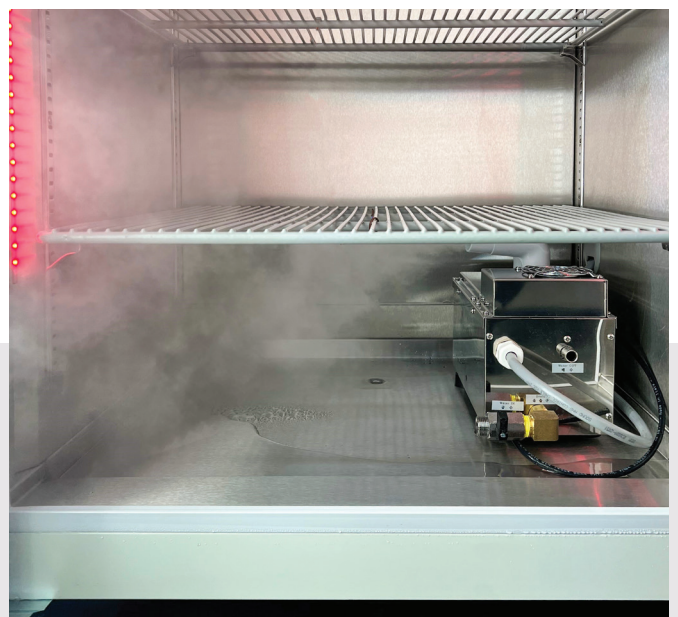
Ultrasonic humidity control box
