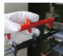
For clamping around the target busbar
