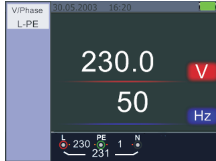
Figure 5.2.7.2 Screen while measuring Voltage and Frequency
