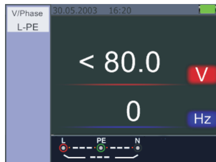
Figure 5.2.7.1 Standby screen for the Voltage and Frequency
