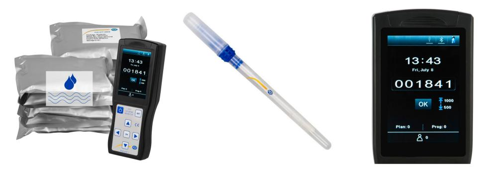
PCE-ATP 1 KIT3 Food & Hygiene ATP Testing Meter / Fast hygiene measurement / Simple sampling / USB and Bluetooth printer interface / Self-calibration at power up
