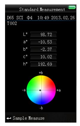
A reading which has been determined by using the "Standard Measurement" automatically serves as a reference value.
