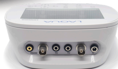
Multi-parameter meter with dual channel input
