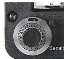
On the sensitivity selection switch is a LOCK lever. This allows a user to lock the sensitivity selection and thereby prevent it from being moved inadvertently. To lock the sensitivity selection, rotate the lever clockwise; to release the lock, rotate the lever counter-clockwise.
