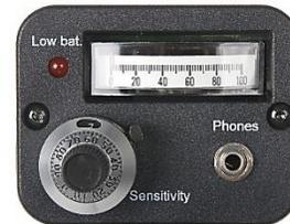
**ANALOG METER.** This ballistic meter has intensity increments of from 0 to 100. The 50 divisions reflect intensity changes only: the more intense the ultrasonic signal, the higher the reading.
