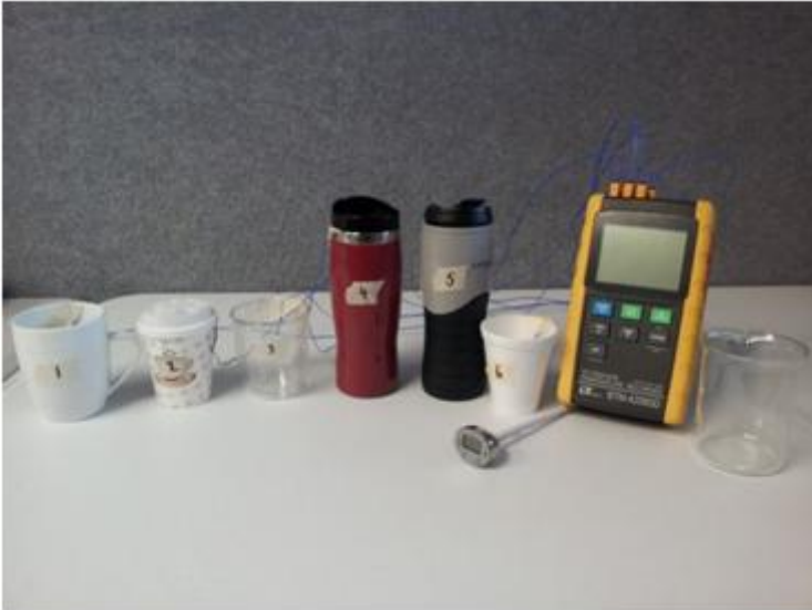
Figure 1: All cups with thermocouples installed ready for testing to begin
