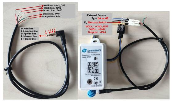
Above is connection to a mercury switch, rotate the mercury will generate interrupt. LHT65 will detect it and send an uplink package to sever. User can also connect PA9 and PA10 together, with these two pins shortcut, LHT65 will know if the probe is connected well in the socket.
