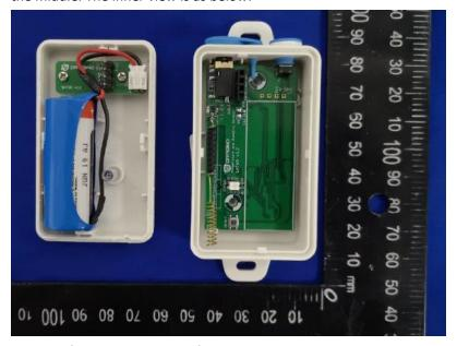
User can find the same type of battery to replace. Or can order our battery replace kit, which include the enclosure and the battery, the part number is LHT65-BAT-CA.
