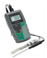
The EC-PH5/02K Ecoscan meter, is a high quality and professional pH and temperature meter, which has an external probe for easy sampling. The meter reads pH within the range 0-14pH with and accuracy of +/- 0.01pH, temperature can be measured between  $0^{0}$ C and  $100^{0}$ C. This meter is supplied with buffer solutions pH4 and pH7 as well as deionized water for rinsing. The meter has a protective rubber shield to protect it from accidental knocks; it is a robust and high quality meter.
