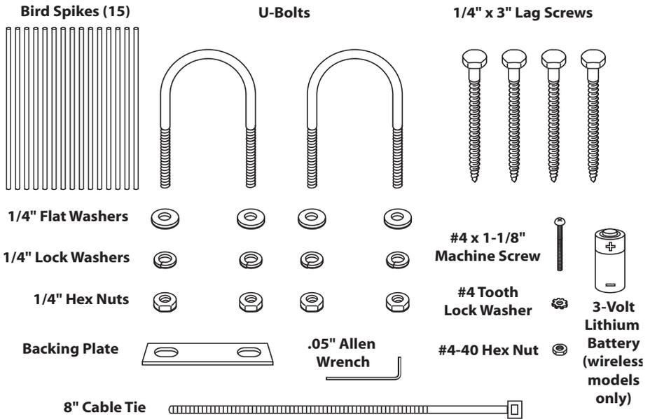
Some of the hardware is optional based on how the ISS is assembled and installed.
