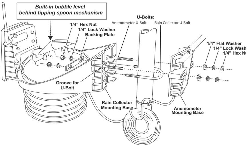
When installing the ISS on a pole, the rain collector / radiation shield section of the ISS and the anemometer can be mounted together as a single unit, or the two sections can be mounted separately.
