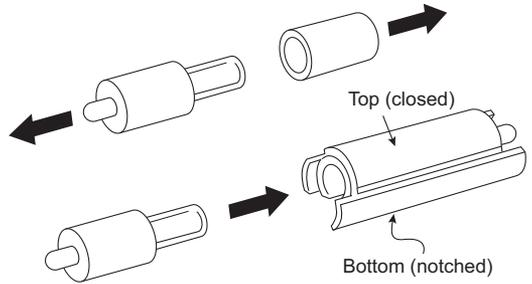
6. Insert the metric adapter and magnet between the arms of the spoons, with the top (solid side) of the metric adapter facing up.
