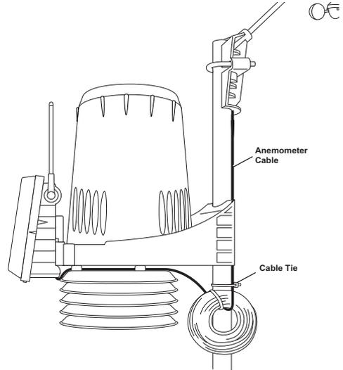
Keep the anemometer cable coiled if possible during the ISS and anemometer assembly so that it is easily stowed once installation is complete.
