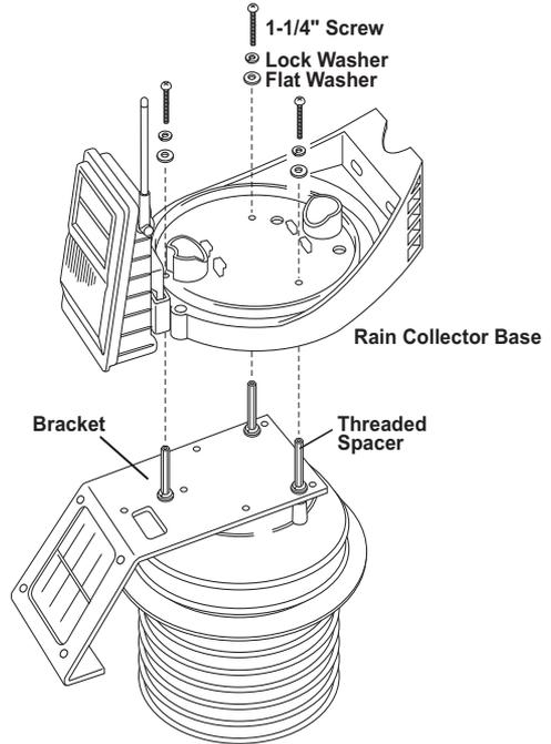
5. Unscrew the three threaded spacers holding the solar bracket and radiation shield together.
