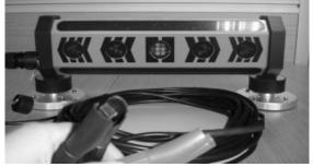
4.2. Charge the inside rechargeable battery by the special 240 V charger, the charging time is 6 hours.
