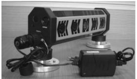
4.3. The MR360 is supplied with remote display, which can be connected to the receiver by the special cable. By installing the remote display inside the cabin this will enable you to view the indicating arrows directly rather than always focusing your eyes on the machine's cutting edge, which makes it possible to locate the receiver higher than the cab to prevent laser beaming blocking and to ensure 360 degree reception.
