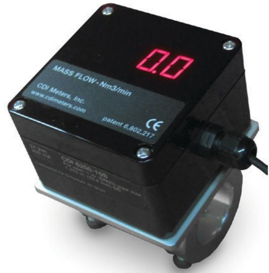
The flowmeter clamps onto a pipe, with two flow-sensing probes projecting into the pipe through 3/16-in. drilled holes. It seals directly to the pipe; no cutting or welding is required for installation. Because each flowmeter is made and calibrated for a specific size of pipe, the display indicates flow directly, with no setup or adjustment.
