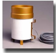
Rainfall: Tipping bucket electronic rain gauge composed of a complex spun collector funnel with a knife edge that diverts the water to a tipping bucket mechanism. For each tip, a magnet causes an electronic pulse to be recorded. The rainfall sensor is completely automatic and requires no servicing.
