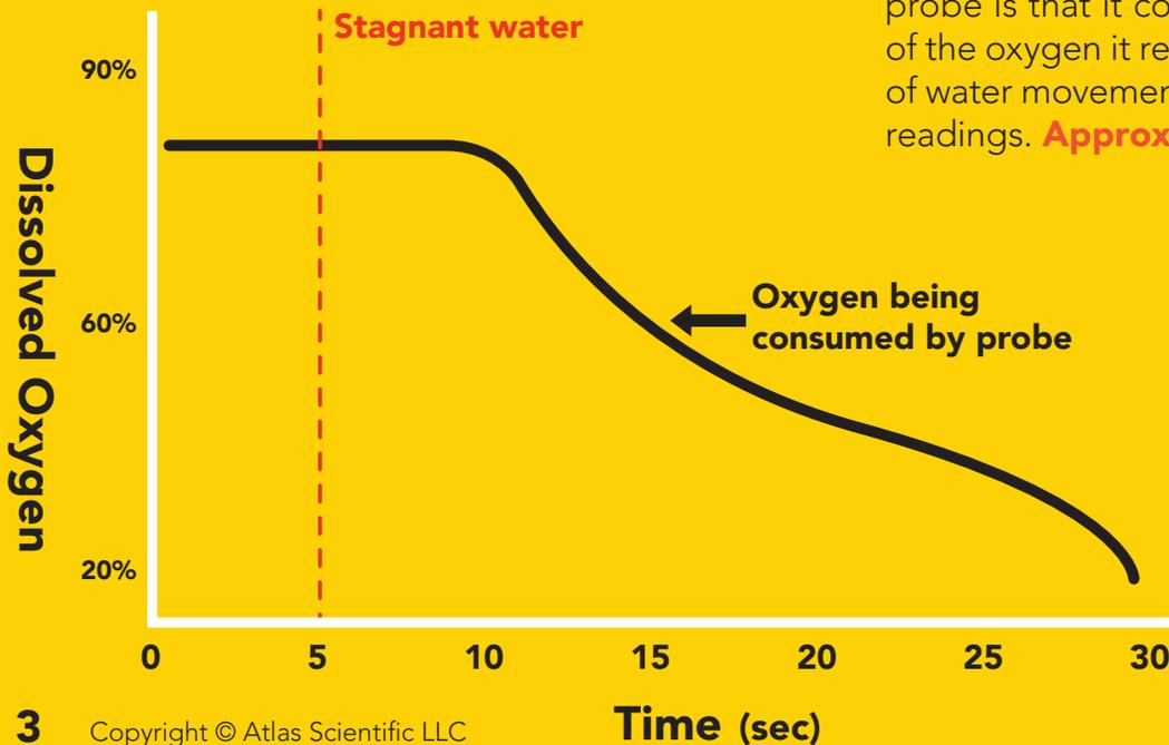
One of the drawbacks from using a galvanic probe is that it consumes a **VERY** small amount of the oxygen it reads. Therefore, a small amount of water movement is necessary to take accurate readings. **Approximately 60 ml/min.**
