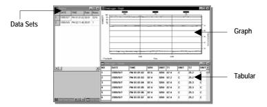
Data Sets Window – Display how many data sets were loaded and the detail information for each data set (start date, start time, recording rate and data length), and you can click at any data set to choose the set for graph and tabular Window.
