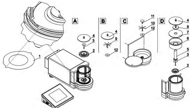
**Caution!** Make sure there is no protective sticker 1 while carrying out the measurement (see the above diagram). It is obligatory to remove the sticker prior chamber assembly.
