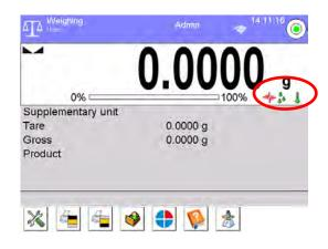
Vibrations are signalled by a respective pictogram displayed in the weighing result window.
