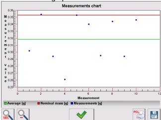
14. Measurements graph with thresholds:
