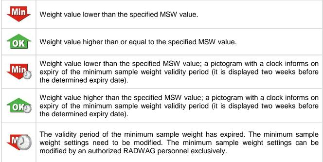
**Caution!** If more than one reference tare value is programmed (with corresponding minimum sample weight mass) then the indicated value automatically moves to a range corresponding to the weight of the tared container. At the same time the required minimum mass is changed.
