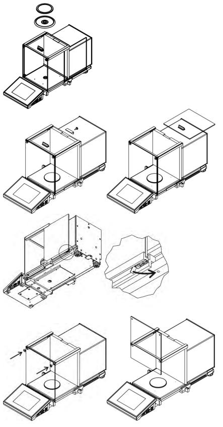
Remove the weighing pan and draft shield. Clean the components when detached. With this your balance mechanism is protected against accidental damage.
