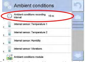
By default the interval is set to 10 min, this value may range between 1 min - 60 min. Record analysis allow the user to select the most optimal time of the day for the measurements performance, i.e. time when the environmental conditions influence the vibrations the least. Mind that there are places where the most convenient working conditions occur after-hours.
