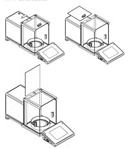
Undo and remove top pane protection, next slide the pane out of a guide bar.
