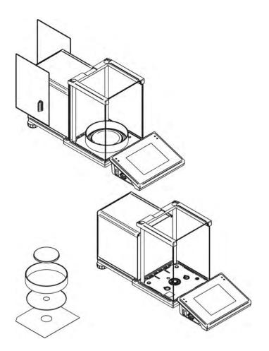
Remove the left and the right side pane. The side panes are not interchangeable therefore it must be remembered which is left, which is right. Upon cleaning procedure completion, the panes must be installed on the correct side.
