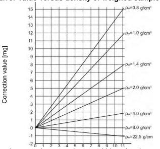
The graph presents correction values for versus the density of weighed load, assumption that air density is constant and equals 1.2 kg/m³ is taken.
