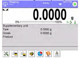
Upon pressing vibrations pictogram, window with current values measured by sensors is displayed. Displayed vibrations value (IS V) is the effective value registered within the most recent 2 seconds.
