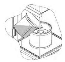
Prior pipettes calibration, distilled water must be poured into the evaporation ring, the amount of water cannot exceed 2/3 of the ring height. The set may be operated after about an hour – this period of time is required for humidity stabilisation. Remember to control the level of distilled water – surface of the vessel has to remain covered with it. Excess of water may be removed by means of an automatic aspirator or an external pipette.
