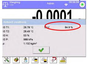
Vibrations are recorded in the database, this allows to analyse history of ambient conditions quality.
