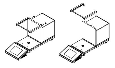
Undo the screws protecting the top frame, next remove it.
