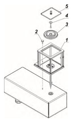
Take all the components from the packaging. Install the anti-draft chamber (1) and screw it to the base using bolt (2).
