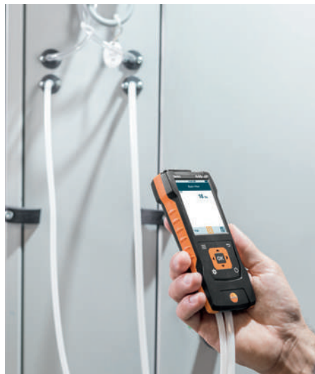
With the testo 440 dP model, incl. differential pressure sensor, you can ensure that the filters in air conditioning systems are working properly and no contamination in the outdoor air gets into the indoor air.
