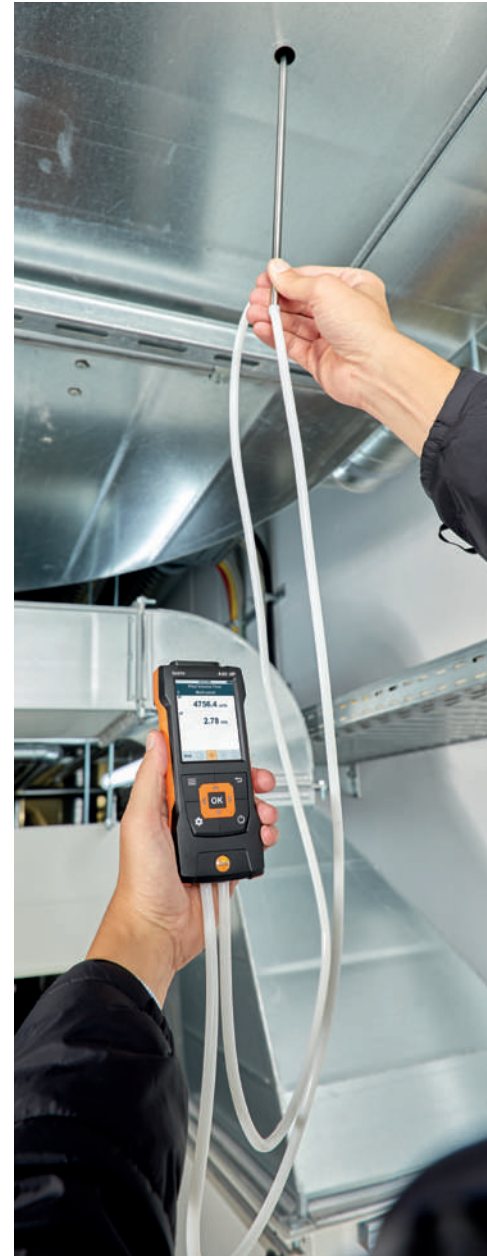
For measuring the volume flow in the case of high flow velocities or heavily contaminated flow, we recommend the testo 440 dP and a Pitot tube.
