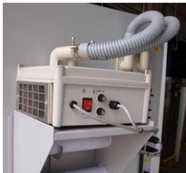
Ultrasonic humidity control box
