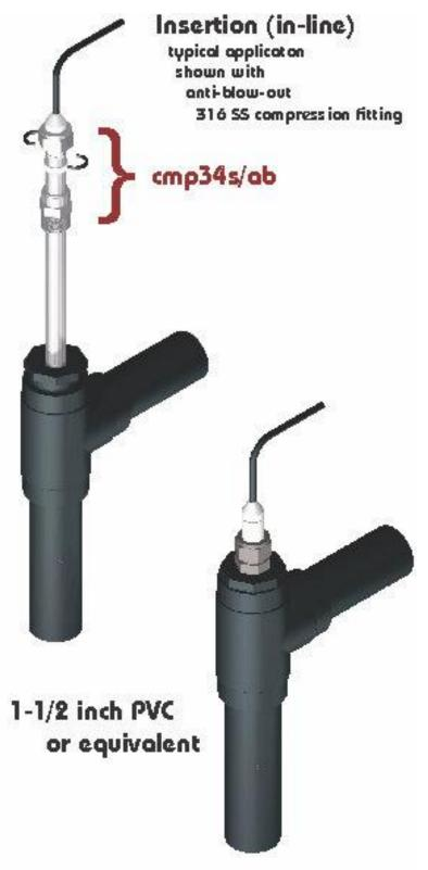
The sensor/transmitter can also be implemented as shown here with the cable for in-line mounting on a skid-mount system. This uses the cmp34/s ant-blowout system fitting to prevent accidental blowout in such applications
