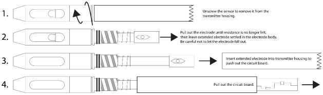
Pay attention to which end was facing the cable to allow for proper alignment when reinserted.
