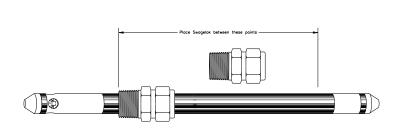
indents on the housing with the threads directed toward the sensor end of the sensor/transmitter. For the most accurate operation of temperature and temperature compensation, it is recommended that the fitting be positioned closer the cable end of the to sensor/transmitter. Tighten the fitting until it firmly grasps the
