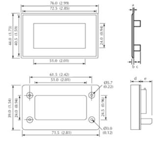
Panel cut-out 72 x 40 (2.83 x 1.57) Maximum panel thickness 3mm (0.12).
