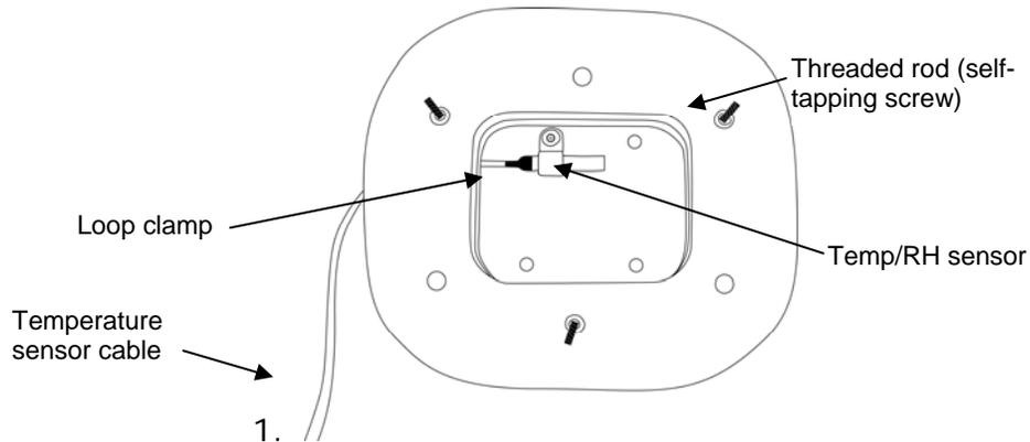
Figure 2: Temperature sensor inside solar radiation shield
