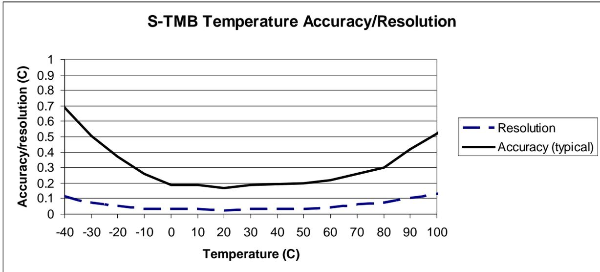
Figure 1: 12-Bit Temperature Smart Sensor Accuracy and Resolution
