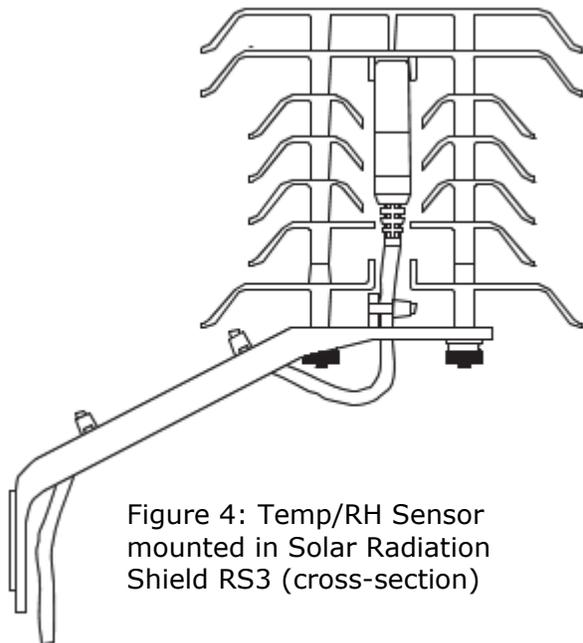
Figure 4: Temp/RH Sensor mounted in Solar Radiation Shield RS3 (cross-section)
