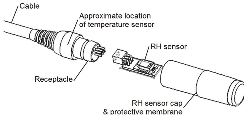
4. Push gently but firmly to install the new sensor (Onset part # HUM-RHPCB-2) **in the same orientation.**
