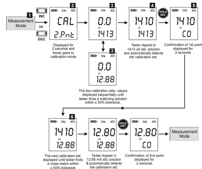
Figure 7: Two-point automatic calibration sequence for ECTestr11
