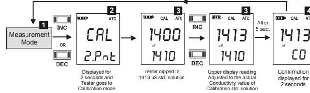
Figure 8: One-point manual calibration sequence for ECTestr11+
