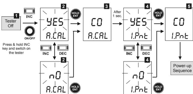
Figure 6: Selecting auto calibration & 1-point calibration for ECTestr11+
