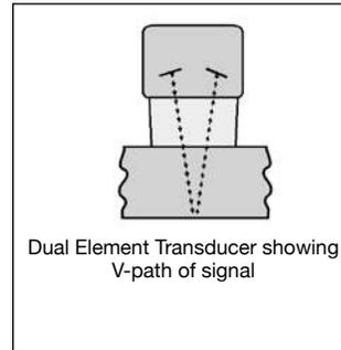
Dual element transducers are normally used in pulse-echo mode for finding defects, and in echo-echo mode for through coating measurements.
