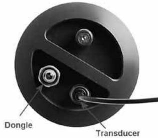
**NOTE:** There is no polarity associated with connecting a dual element transducer. If a single element membrane style is connected, the dongle ‘must’ be plugged into the connector labeled in the diagram above, in order for the TI-UMX2 to ‘auto identify’ the single element probe type.
