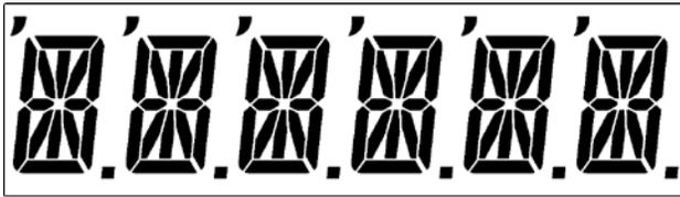
The TI-UMX2 is equipped with two segmented LCD displays that are used for entirely different purposes. The 6 Character display above, is used for all the menu options and any text to control the overall operation and functionality of the TI-UMX2. Since the TI-UMX2 has the ability to store measurements, this display is also used to view and move to specific cell/storage locations in the grid storage structure of the gauge.
