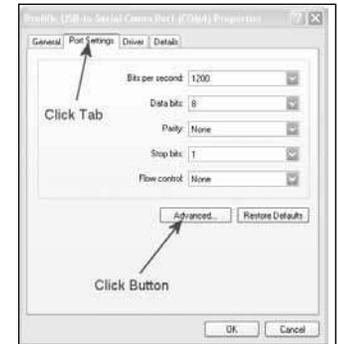
7. Assign a com port 1-4 to the device, and click OK to set the port.
