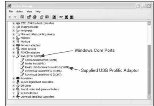
5. Open Windows® 'device manager' and click the plus sign next to PORTS, in order to display the complete list of all com ports in use. Look for the device named "Prolific USB-to-Serial to determine the current port that windows® has assigned the device.
