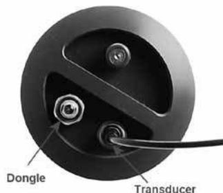
1. Connect the probe to the TI-UMX2.
