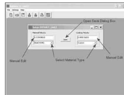
4. Once the material and or coating velocities have been set, click the SAVE button in the setup dialog box, to display the SAVE dialog box.
