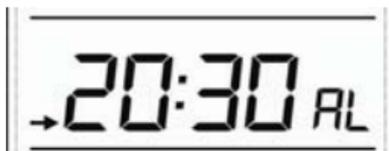
1. While in normal time display mode, press the CH/+ key twice to display alarm time
