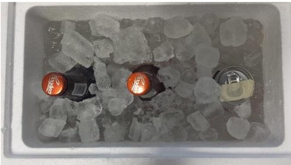
Figure 1: Foam esky with salt/ice slurry with beers and loggers submerged
