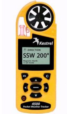
For years our customers have been asking for wind direction along with wind speed. New for 2007, the Kestrel 4500 does just that with its built in digital compass. But it doesn't stop there. It also calculates crosswind and headwind/tailwind with reference to a user-set target heading, and stores the information along with all the other environmental readings in its 1400 data point memory.
