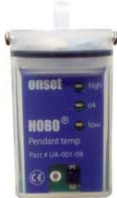
A miniature one-channel temperature logger, this model is waterproof and value-priced for short-term shipping applications or year-long remote deployment. Logger alarm LEDs flash if temperatures have exceeded user-set levels and delay options, and provide visible verification that temperatures have been within the desired range throughout deployment. This 8K model stores approximately 6.5K of 10-bit temperature readings.
