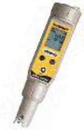
The EC-PHTESTR20 is a high quality, waterproof (IP67) pH pen tester. This unit allows for automatic temperature compensation although it does not display the temperature. This unit is durable and good quality and reasonably priced, it is able to measure pH between 0pH to 14pH with an accuracy of +/- 0.01pH.
