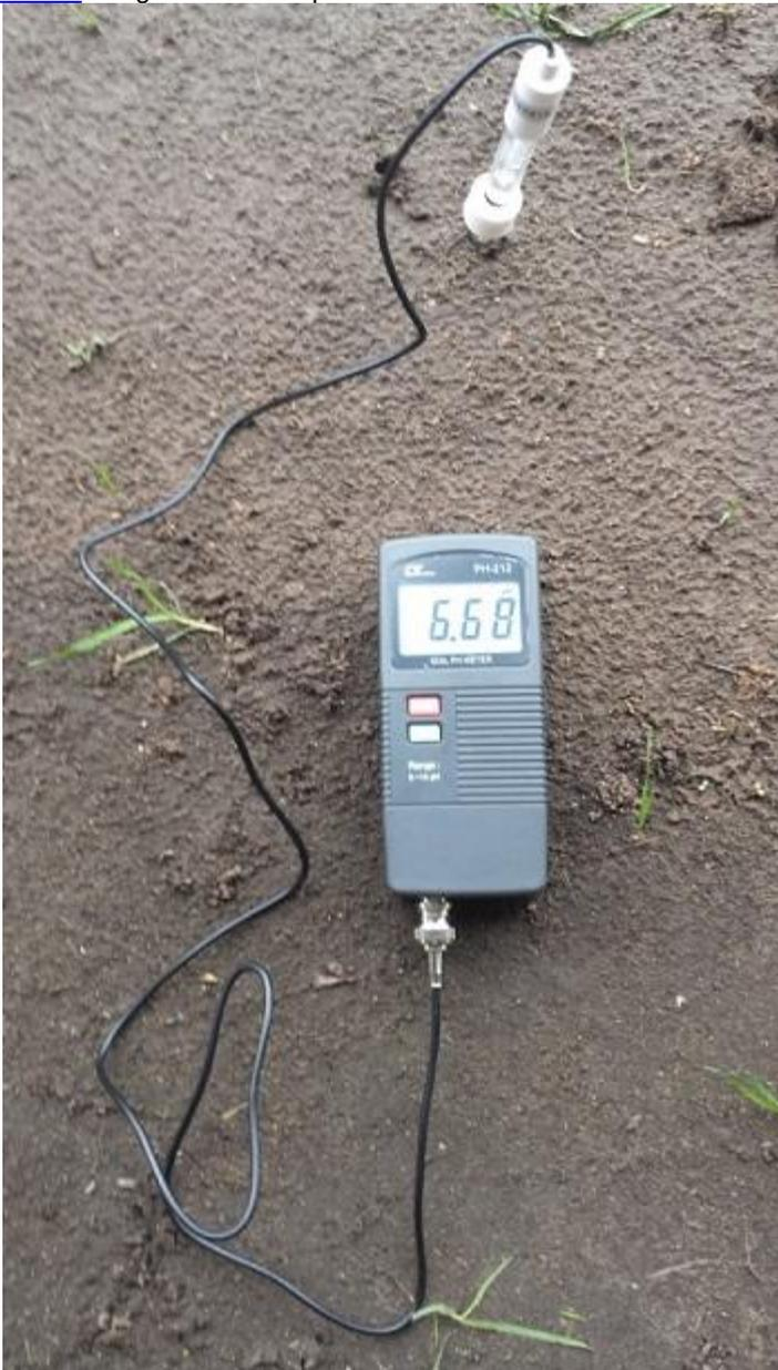
For this test the soil sample was prepared as for the [ICZD06](#). The spear tipped electrode was then carefully inserted into the soil ensuring good contact with the soil. The pH of the soil was then read off the digital display once it had stabilised which typically took 5-20 seconds. Prior to each test the unit
