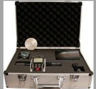
The [IC-Window-Kit](#) - Self Certification Kit from Instrument Choice contains everything you need to test windows and screens to the new BCA codes for children's safety. The kit is designed to replicate the force a young child may put on a window or screen, with the 125mm bullet shaped probe replicating a child's head and the 125mm pressure plate replicating any flat surface.
