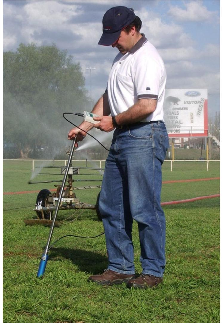
The MPKit measuring surface volumetric moisture content
