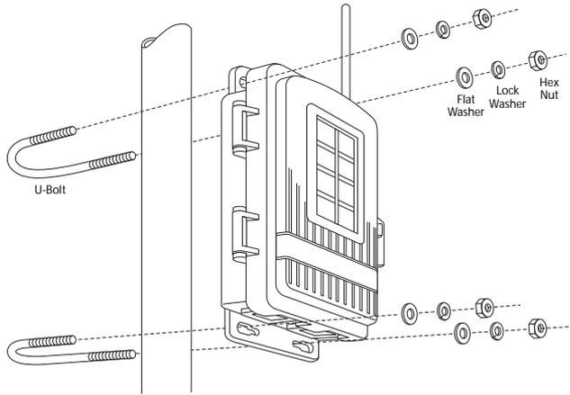
Note: Remember to position the shelter so the solar panel has maximum exposure to the sun.
