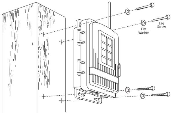
Note: Remember to position the shelter so the solar panel has maximum exposure to the sun.
