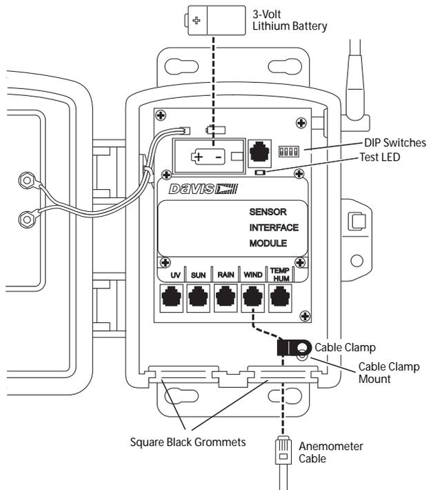
3. Plug the end of the anemometer cable into the receptacle labeled WIND on the SIM.
