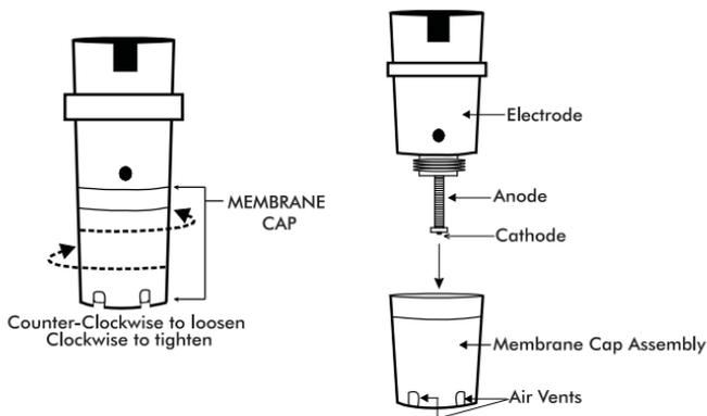
4. Rinse the cathode and anode with deionized water.
