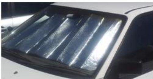
Figure 3: Vehicle with reflective shield fitted to front windscreen
