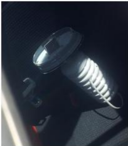
Figure 1: Radiation shield and data logger positioned in rear seat.
